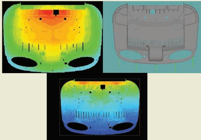
Figure E (left): Gate location and orientation. Figure F (right): Gate location and orientation. Figure G (bottom center): Surface color map: fill pattern – blue = early fill, red = late.
